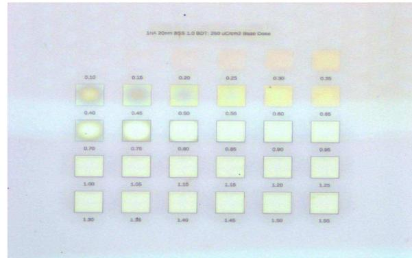
With DisCharge, no charge accumulation is observed. The structure appears as expected with no hard to PDMS from sudden dielectric breakdown.
